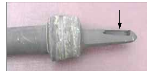
Thermowell Boss Erosion
