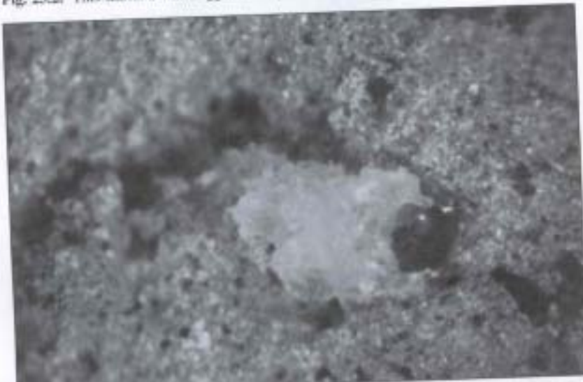
Fig. 23.2. This shows a white eggshell shape of flux around some shrinkage porosity.
