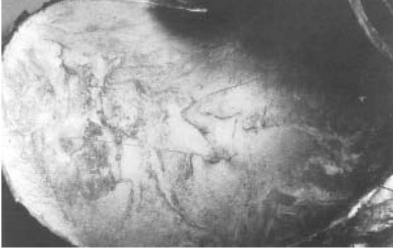
18-1: typical stained casting
