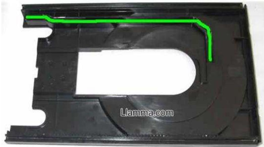
Now with the tray completely out move the actuator so the laser assembly is all the way at the bottom of its travel, line up the tray so the nub fits back in the tray and simply push the tray back in the rest of the way. Reassemble the drive and test!
