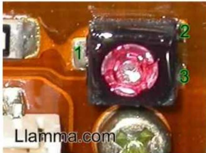
Scrape away the epoxy on the screw, not always an easy task and probably the most likely chance to irreparably damage your DVD. The epoxy sticks well and you need to pick at it hard to get it off, I use an X-Acto knife. Attempt to slice across the top of the screw until you expose silver across the surface then use a pick to remove the epoxy in the center of the screw.
