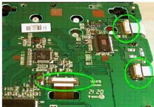
To remove them be sure to dislodge the wedge that holds them in place. Start on one side and then the other. This can easily be accomplished with a fingernail or delicately with a screw driver.
