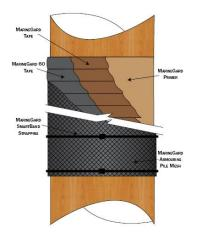
The MarineGard Series 60 System is designed to protect
